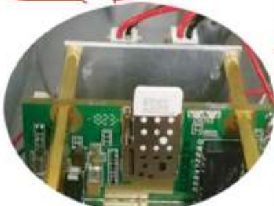
SIM card type is Nano SIM(12.3mmx8.8mm)
